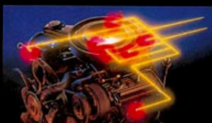
For 1985, Monte Carlo has a new standard Electronic Fuel Injection 4.3 Liter V6 engine that uses the same cylinder bore and stroke as Corvette for a 13.2% displacement increase.
