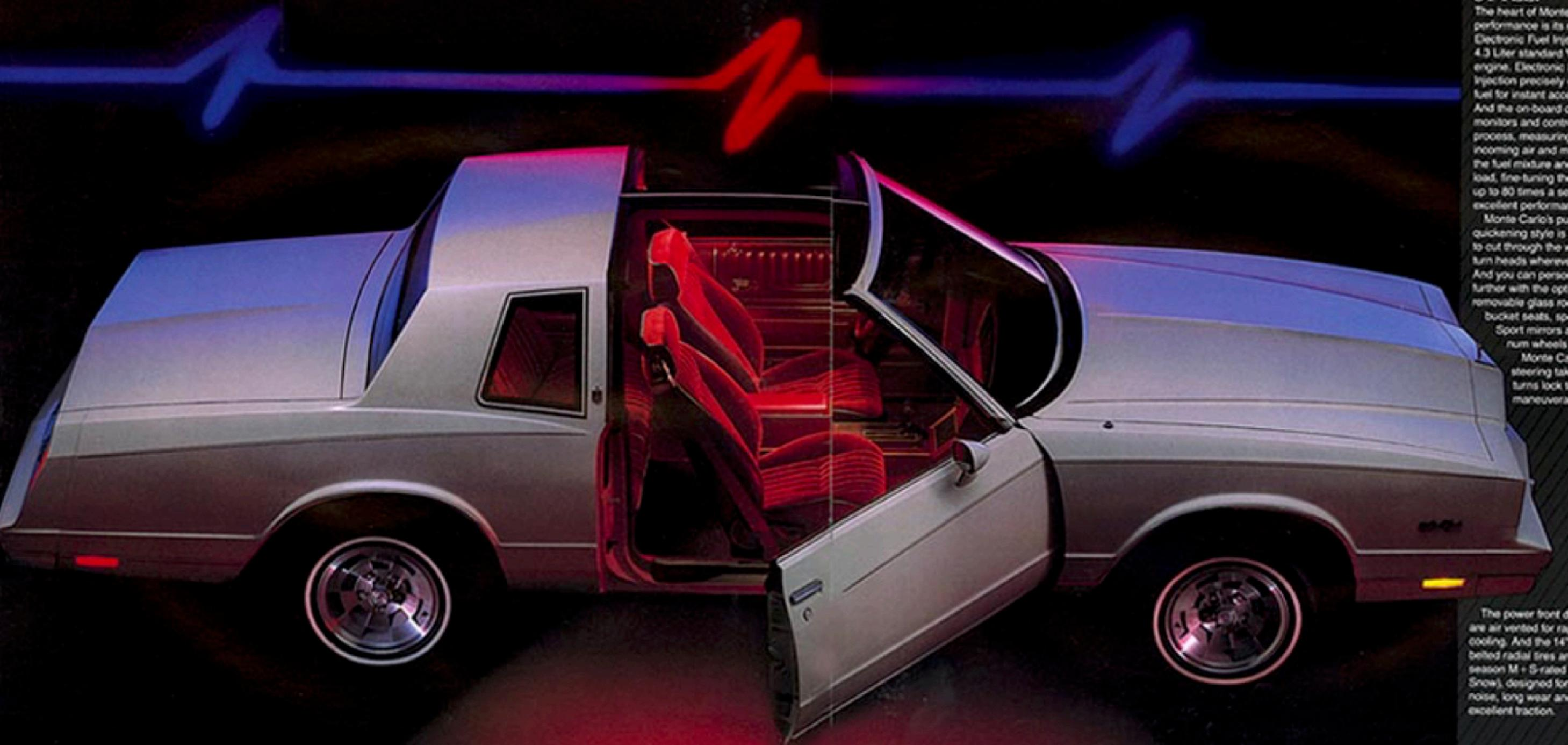
The power front disc brakes are air vented for rapid cooling. And the 14" steel-belted radial tires are all-season M+S-rated (Mud and Snow), designed for low noise, long wear and excellent traction.
