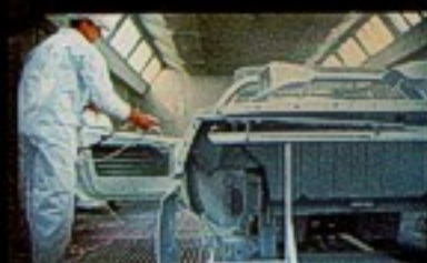
Clean-room environment is a key part of the paint process.
