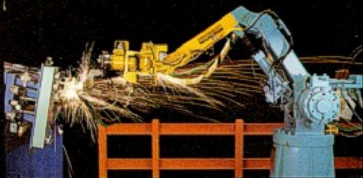
Uniframe components get additional precision robot welds.
