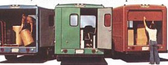
models, with wider doors available. All models feature windows in each rear door. Overhead rear doors, available by special order on all models, are especially useful for backing right up to loading docks. Also for easy access, wraparound double doors are available on all models. Wide doors fold back flush with side panels, with width keyed to body size.
