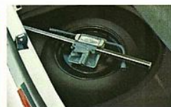
Compact Inflated Spare. Designed to save space and weight. Comes fully inflated, ready to use for emergency purposes.
