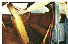
Inertia-Type Seat Back Latches. No exterior latches to grope for. Front seat backs fold forward at a touch, yet latch automatically in sudden stops. Two-door models only.
