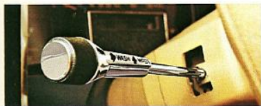
Column-Mounted Control. Puts turn signals, headlight dimmer, windshield wipers and washers in one column-mounted switch for fingertip control.
