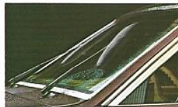
Intermittent Wiper System. Varies the windshield wiper cycle to adjust for heavy downpour or light mist.
