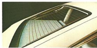
Electric Rear Window Defogger. Electric element helps keep rear window free of mist and frost silently and without drafts.
