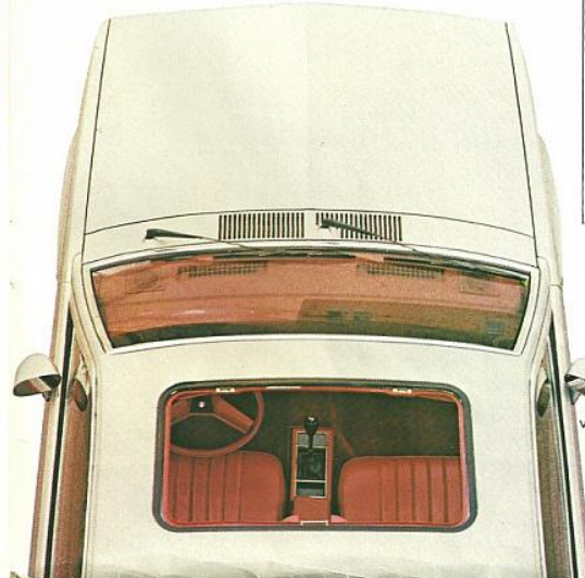
Removable Sun Roof. A refined design with front-hinged glass panel. Pops up for ventilation or can be completely removed. Handy storage bag included.
