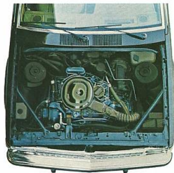
2.8 Litre V6 Engine. A totally new engine designed for the 1980 Chevy Citation. Features compact design with aluminum inlet manifold, water pump housing, engine front cover and carburetor. Strong cast-iron cylinder block and heads, yet is relatively light in weight.
