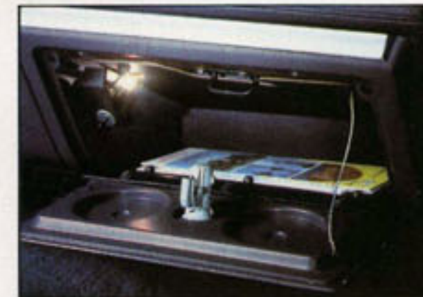
AUXILIARY LIGHTING. Includes: underhood, glove compartment and courtesy lights, right front door dome light switch on Scooter, rear compartment light and switch, headlight warning buzzer.
