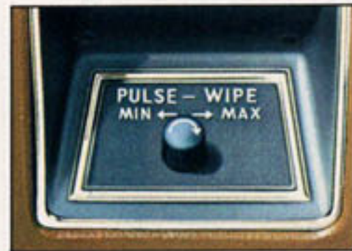
INTERMITTENT WINDSHIELD WIPER SYSTEM. Lets you adjust wipe cycle from 1/2 to as long as 20 seconds.
