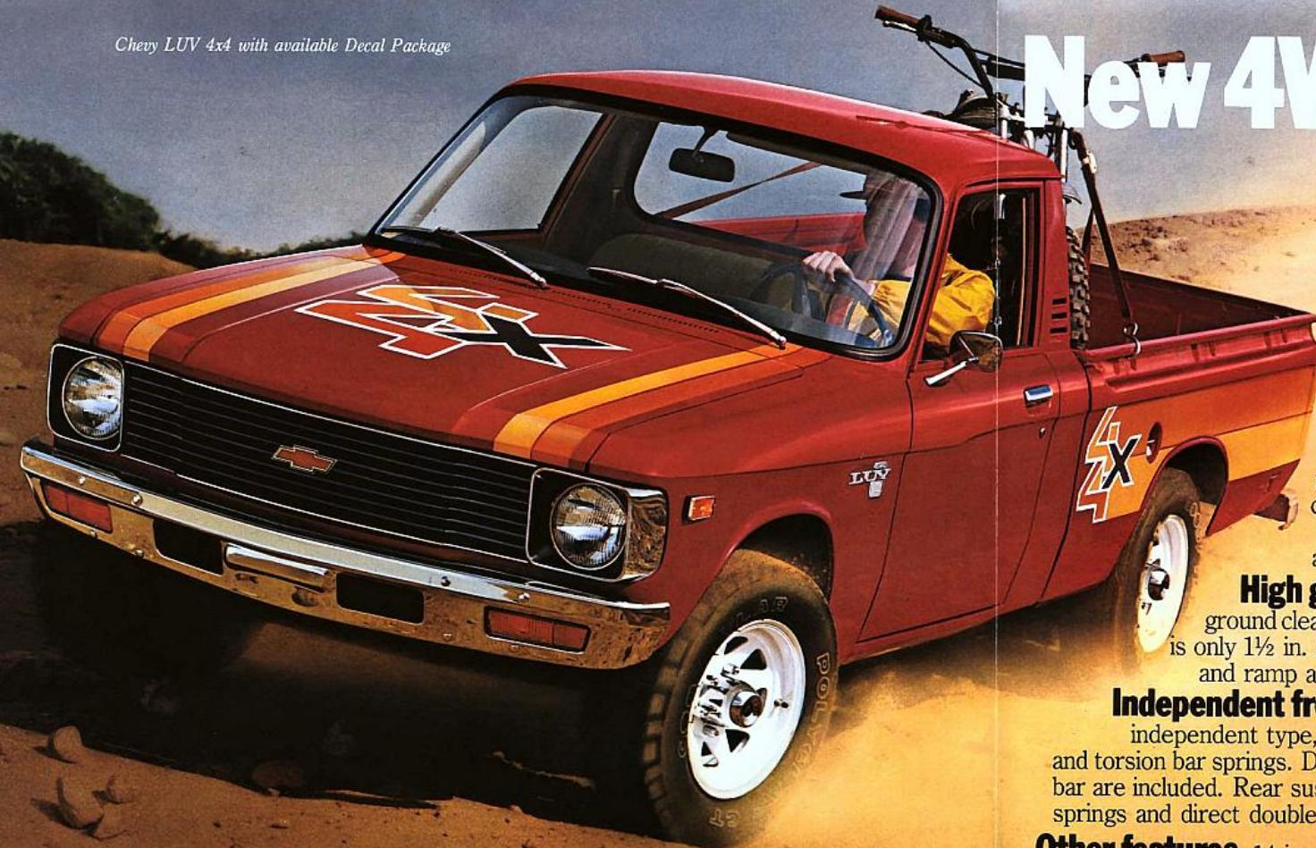
A great way to get into the back country. Light, nimble Chevy LUV 4x4 has a 4-speed, fully synchronized manual transmission with a choice of Hi and Lo 4WD positions. The transfer case is combined with the transmission in a single unit and each is operated by a separate shift lever. Manual locking hubs are an additional standard feature of the system.
