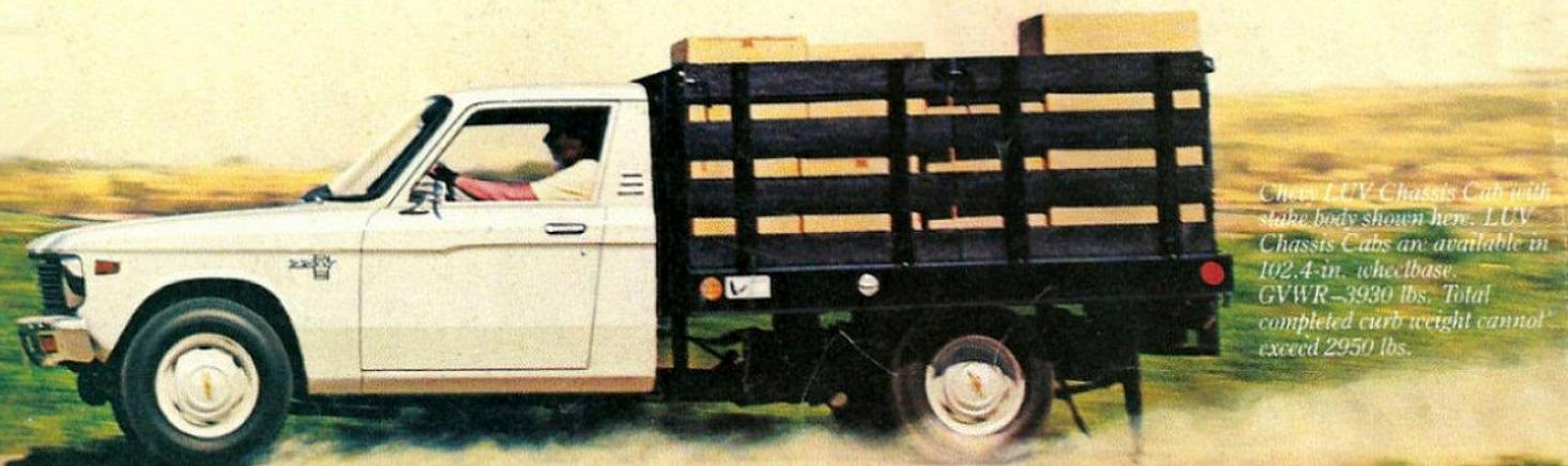
Chevy LUV Chassis Cab with stake body shown here. LUV Chassis Cabs are available in 102.4-in. wheelbase. GVWR—3930 lbs. Total completed curb weight cannot exceed 2950 lbs.
