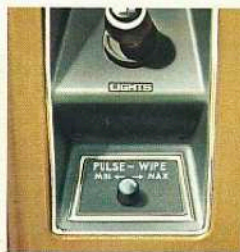
Intermittent Windshield Wiper System. Lets you adjust wipe cycle from 1/2 to as long as 20 seconds.
