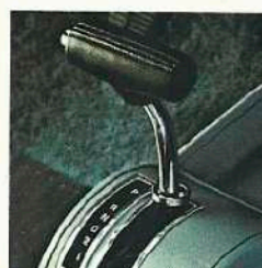
Automatic Transmission. Three speed ranges. May be shifted manually.
