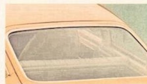
ELECTRO-CLEAR-REAR WINDOW DEFOGGER. Dash-mounted on-off switch, controls electric heat to defog rear window. Time delay switch automatically shuts off defogger (in case you forget) to prevent excessive battery drain.
