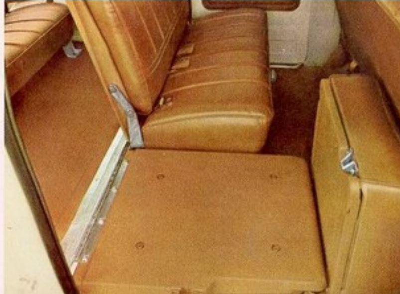
Cushion unlatches and folds forward. Backrest unlatches and folds down.
