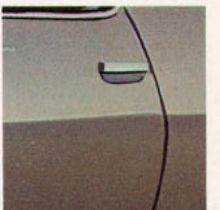
**Flush-mounted door handles.** Just lift to open. Convenient, easy-to-grasp operation.
