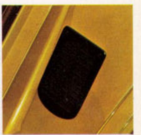
**New Flow-Through Power Ventilation System.** The three-speed blower brings in outside air without the need to open a window. It may be blended with heated air as required. In addition, an engine temperature sensor will delay operation of the blower in "low" position until the engine warms up, to operating temperatures.
