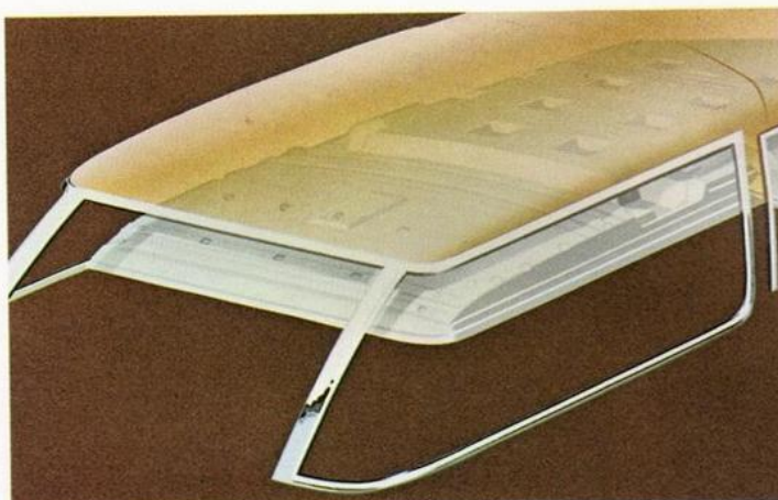
Double-panel roof structure. Two layers of steel overhead for extra strength and extra quiet.
