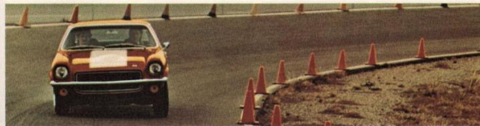
Vega has a wide stance and a low centre of gravity for stability.
