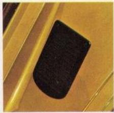
**New Flow-Through Power Ventilation System.** The three-speed blower brings in outside air without the need to open a window. It may be blended with heated air as required. In addition, an engine temperature sensor will delay operation of the blower in "low" position until the engine warms up, to operating temperatures.
