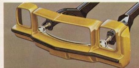
**Laguna Front Bumper System.** This distinctively styled front end nose cone is entirely covered by a resilient, rubber-like material called urethane, which resists
