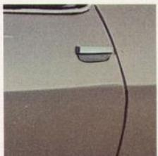
**Flush-mounted door handles.** Just lift to open. Convenient, easy-to-grasp operation.
