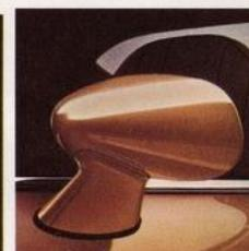
**Dual Sport Mirrors.** Matching body color. Mirror on the driver's side is adjustable without lowering the window, using the remote control knob on the inside door panel. Right-hand mirror is manual. (Included on SS.)
