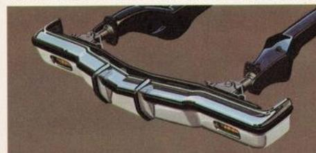
**New Improved Front Bumper System.** This new system retracts on minor impact and hydraulically cushions the shock. (Shown with deluxe bumper styling.)
