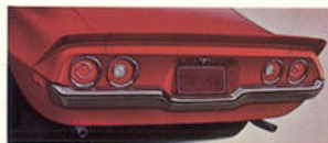
Front and Rear Spoilers. Include lower front spoiler and a special full-width rear spoiler that extends down sides of rear fenders. Both spoilers add to Camaro's handling, especially at highway speeds.
