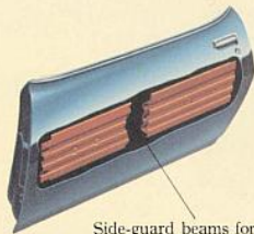
Side-guard beams for side impact protection.
