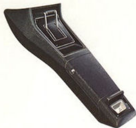
Floor Console. Mounts between front bucket seats. Contains storage compartment, ashtray for rear passengers and houses transmission shift lever when ordered.
