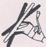
4-speed transmissions. It allows the steering wheel to be adjusted to any of seven different angles by means of a lever on the steering column.
