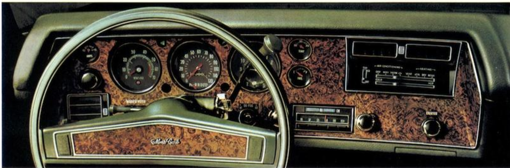
Monte Carlo dash with special instrumentation which includes tachometer plus needle gauges for ammeter and temperature may be ordered. Four-Season air conditioning illustrated is an extra-cost option.
