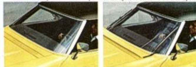
Hide-A-Way windshield wiper-washer system closed . . . and open.
