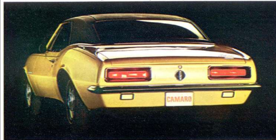
Distinctive rear styling with twin-unit taillight assemblies edged in black, backup lights below bumper and "rs" emblem on fuel filler cap.
