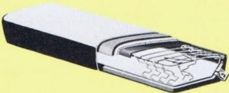
**SPARTAN SEATS** feature a foam rubber pad over flat, coil and S-wire springs for maximum support and comfort. Covering of durable charcoal gray and silver vinyl is standard and \*Custom cabs feature rich pin-seal grain vinyl with nylon-faced pattern cloth. The foam rubber seat option boasts a 6" foam cushion.
