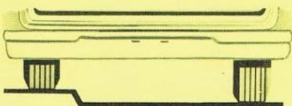
**FREE-STEPPING FRONT WHEEL ACTION** lets each wheel take bumps without passing on the effect to the other, as happens with solid front axles. Cuts road shock and wheel fight. Short-and-long-arm suspension linkage keeps tread width uniform regardless of wheel deflection; tire contact stays at its best under all conditions.
