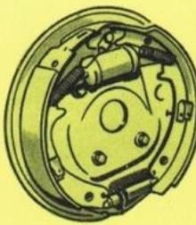
**EXTRA-SIZE BRAKE LINING AREA** means sure, safe stops . . . and lower operating temperatures for longer brake life through slowing the rate of lining wear. Torque action front brakes for added stopping power . . . twin-action rear brakes have dual-acting wheel cylinders.
