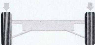
**WIDE-STANCE ROLL STABILITY** is achieved by the independent front suspension design that reduces lean and sway. In an independent system, the effective spring base width equals the full width of the tread . . . nearly doubles the spring base possible with an I-beam axle.
