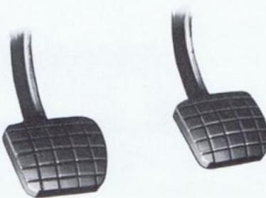
**SUSPENDED PEDALS** add to driver comfort by eliminating openings in the floor to keep out dust, moisture and drafts.
