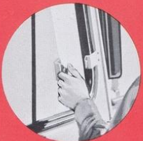
SLIDING WINDOW , located on driver's side, opens easily for ventilating or signaling. When shut, it is leakproof.
