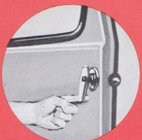
SLIDING SIDE DOORS roll easily on ball bearings and nylon guide bushings. Doors close flush with the exterior of the body.
