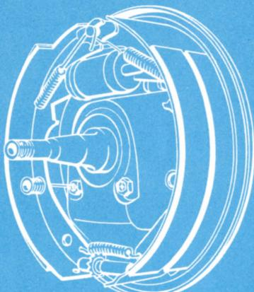
**Air-Cooled Brakes for Safe, Positive Stopping!** Durable, husky brakes are a vital part of sports car driving—and the Corvette's got the brakes to do the job! New slotted wheel discs permit air to cool the innermost areas of the big 11-inch hydraulic brakes, help maintain constant high-brake efficiency and add extra lining life. Brakes are self-energizing with fade-resistant, bonded linings.
