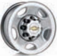
16-inch painted steel wheel, standard on WT models (QB5)
