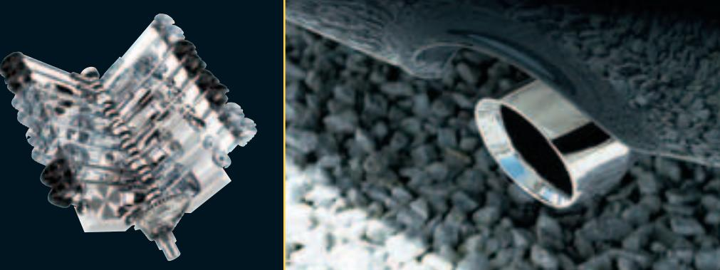
Dual stainless steel exhaust outlets with bright tips provide a performance styling detail.
