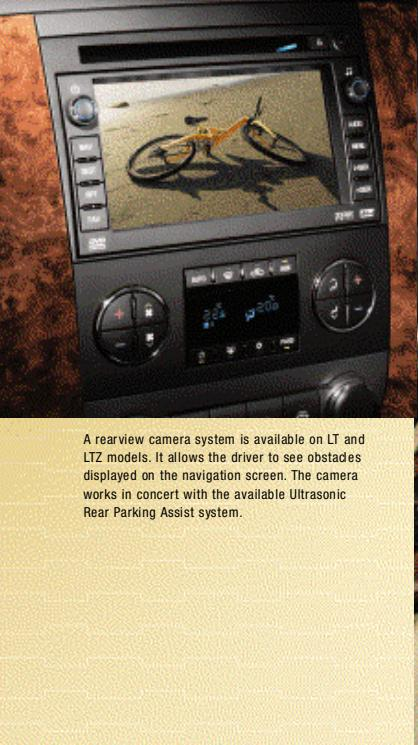
A rearview camera system is available on LT and LTZ models. It allows the driver to see obstacles displayed on the navigation screen. The camera works in concert with the available Ultrasonic Rear Parking Assist system.
