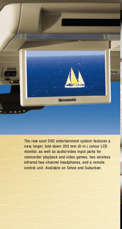
The rear-seat DVD entertainment system features a new, larger, fold-down 203 mm (8-in.) colour LCD monitor, as well as audio/video input jacks for camcorder playback and video games, two wireless infrared two-channel headphones, and a remote control unit. Available on Tahoe and Suburban.
