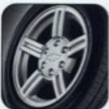
17" x 8" aluminum wheel. Standard on Base and LS models with ZQ6 Sport suspension.
