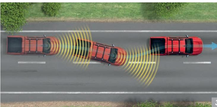
**1. Forward Collision Alert** At speeds of 40 km/h upwards, a camera mounted on the rear view mirror analyzes and evaluates the distance between your truck and the vehicle in front. If you come in too close to the vehicle in front, the system sends out an image and audio alert to the driver.
