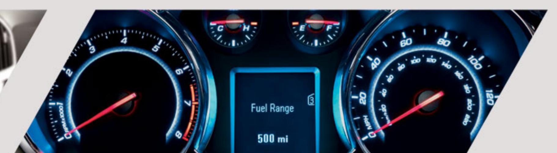
LED illuminated optitron gauges with Driver Information System that provides useful information such as average and instantaneous fuel consumption and remaining fuel mileage
