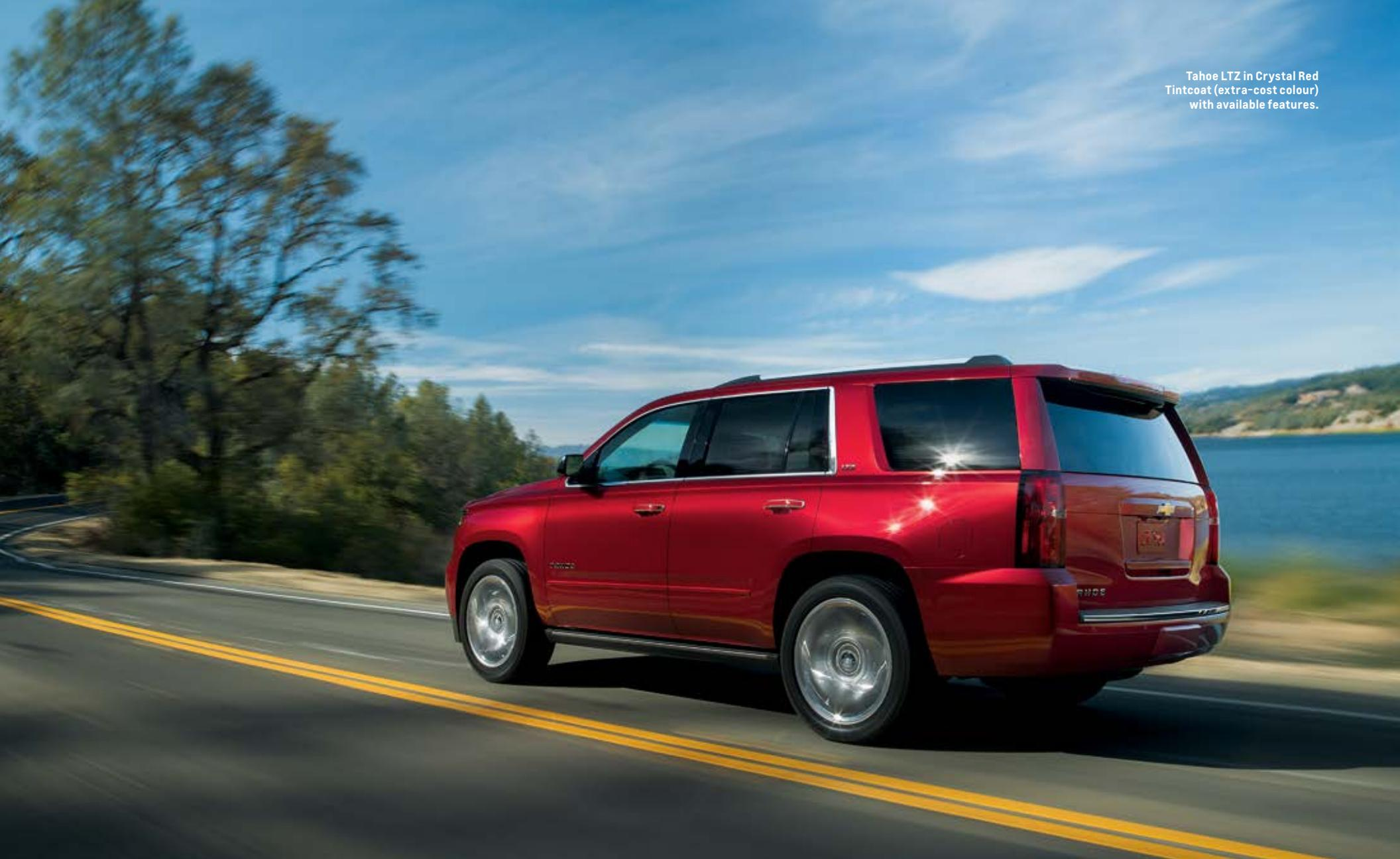
**MAGNETIC RIDE CONTROL.** LTZ models feature Corvette-inspired Magnetic Ride Control<sup>®</sup>, a real-time damping system that delivers a smooth, precise ride by “reading” the road every millisecond and changing damping in just 10-15 milliseconds.
