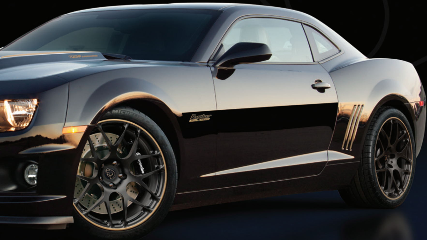
SLP's 700HP Supercharged Panther shown with high-performance RTM hood; carbon fiber and gold accent hood, decklid, and spoiler graphics with 700HP Supercharged cowl graphics; SLP full front fascia with heritage-style front grille and gold Bowtie emblem; 20" x 10" front/20" x 11" rear black satin finish forged wheels with gold accent and Panther center caps; Michelin Super Sport tires; gold rear 1/4 panel gill insert graphics; front splitter; black and gold exterior Panther badges
