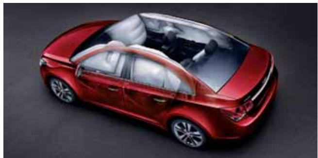
**Ten Air Bags.<sup>1</sup>** Standard on every Cruze, including frontal, front side-impact, roof rail-mounted head-curtain side-impact with rollover capability, outboard rear side-impact, and new knee air bags.
