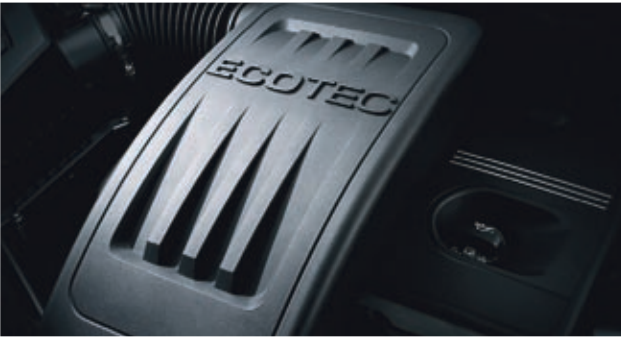
The 2.4L four-cylinder engine produces 182 horsepower at 6700 rpm and 174 lb.-ft. of torque at 4800 rpm.
