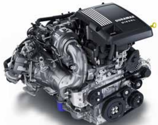
DURAMAX 3.0L TURBO-DIESEL I-6 (LM2) Available on Custom Trail Boss, LT, RST, LT Trail Boss, LTZ and High Country 4x4 models.
