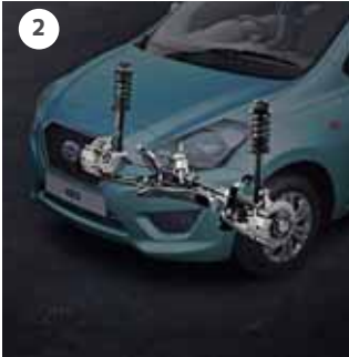
2. Suspension System: A double-pivot front arm enables greater agility, while the tension created by the rough road is absorbed by a high-response damper.
