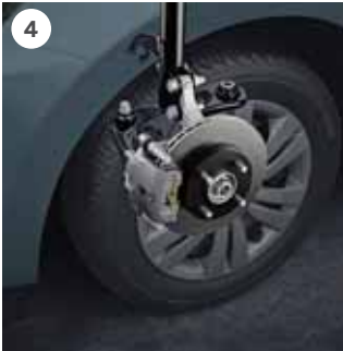
4. Ventilated Disc Brakes: The Datsun GO uses ventilated disc brakes in front. The brake system ensures enduring brakes, which implies more secure and consistent hauling for your car.
