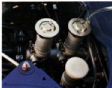
Tandem master brake cylinders for double protection.
