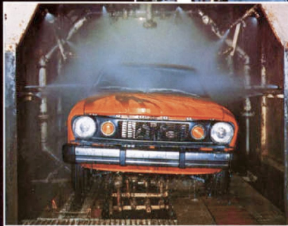
Over three tons of water is splashed on every Datsun to check for leaks.
