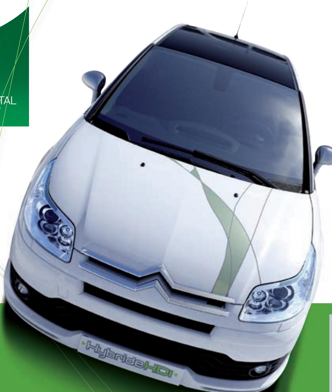
The C4 Hybride HDi (above) combines an advanced 1.6HDi diesel engine with an electric motor.
