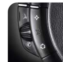
• One of the controls on the left part of the steering wheel allows you to control the air recycling switch<sup>◊</sup> as well as the optional NaviDrive.
