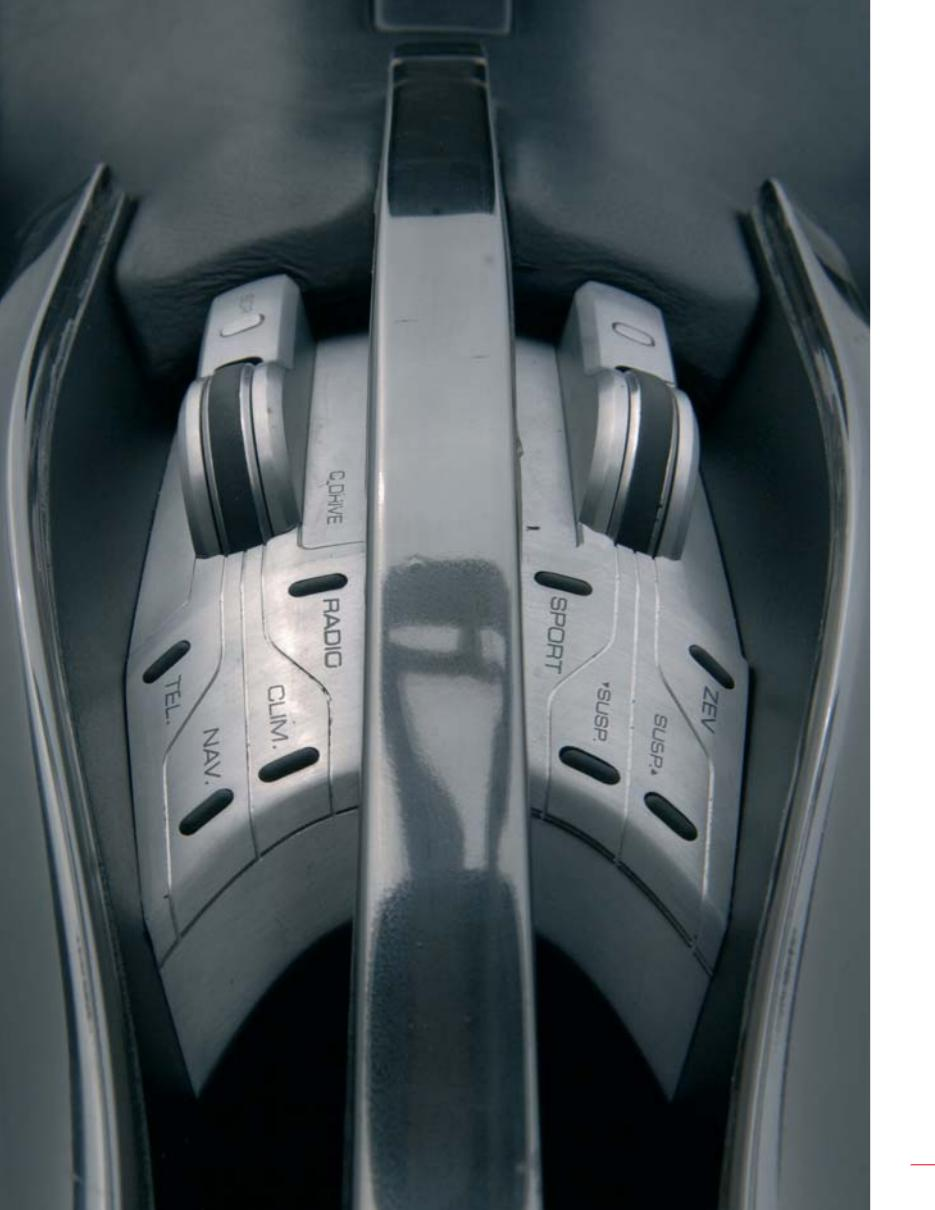
This high-tech equipment perfectly matches the design of the driving position whose original central console is divided by five extensions. Positioned between these extensions are the aluminium gear shift lever and other functions including the navigation system controls; seat, steering wheel and pedal assembly adjustment; boot controls, body height adjustment and the sport mode of the suspension system.
