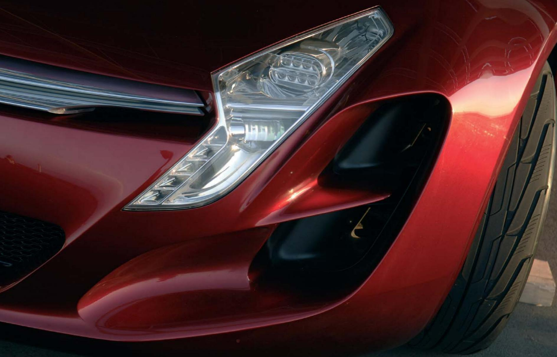
The design lines of C-Métisse also reflect the quest for outstanding aerodynamics, delivering improved fuel economy and lower pollutant emissions while also integrating the latest technological developments. Positioned either side of the double chevron badge on the radiator grille, the headlamps are equipped with a row of LEDs that light up progressively, depending on the steering-wheel angle and vehicle speed. This feature ensures
