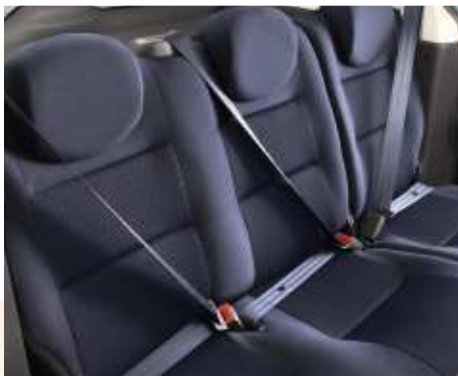
Each of the three rear seats is fitted with a 3-point inertia reel seat belt. Front seat belts are also fitted with pyrotechnic pretensioners and force-limiters for optimal response in the event of impact.
