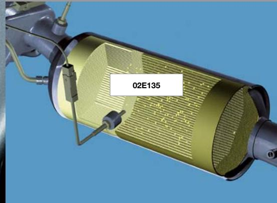
The HDi engine technology on offer in the Citroën C8 is designed to minimise any impact on the environment through lower emissions and superb fuel economy. Certain C8 HDi models can also be fitted with the ground-breaking Particulate Filter System. The filter traps many of the harmful particles responsible for the generation of black smoke and periodically eliminates them by burning them at very high temperatures.
