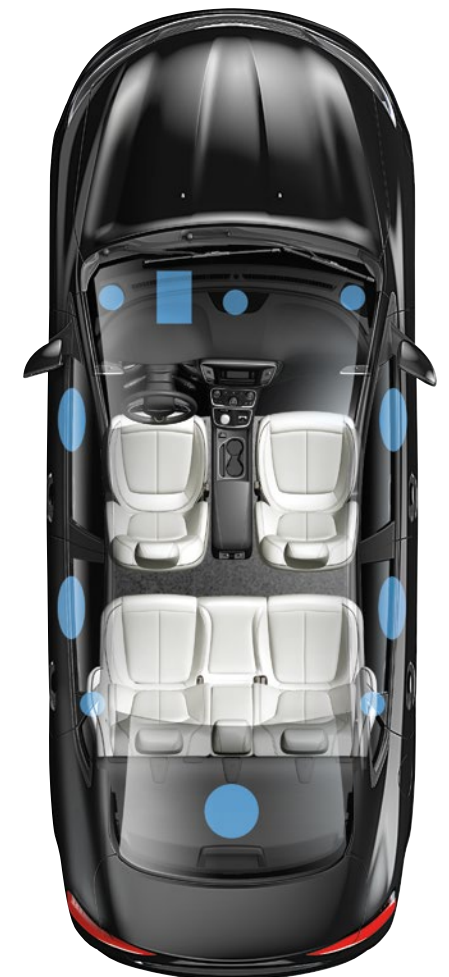
200 Alpine system 10-speaker schematic
