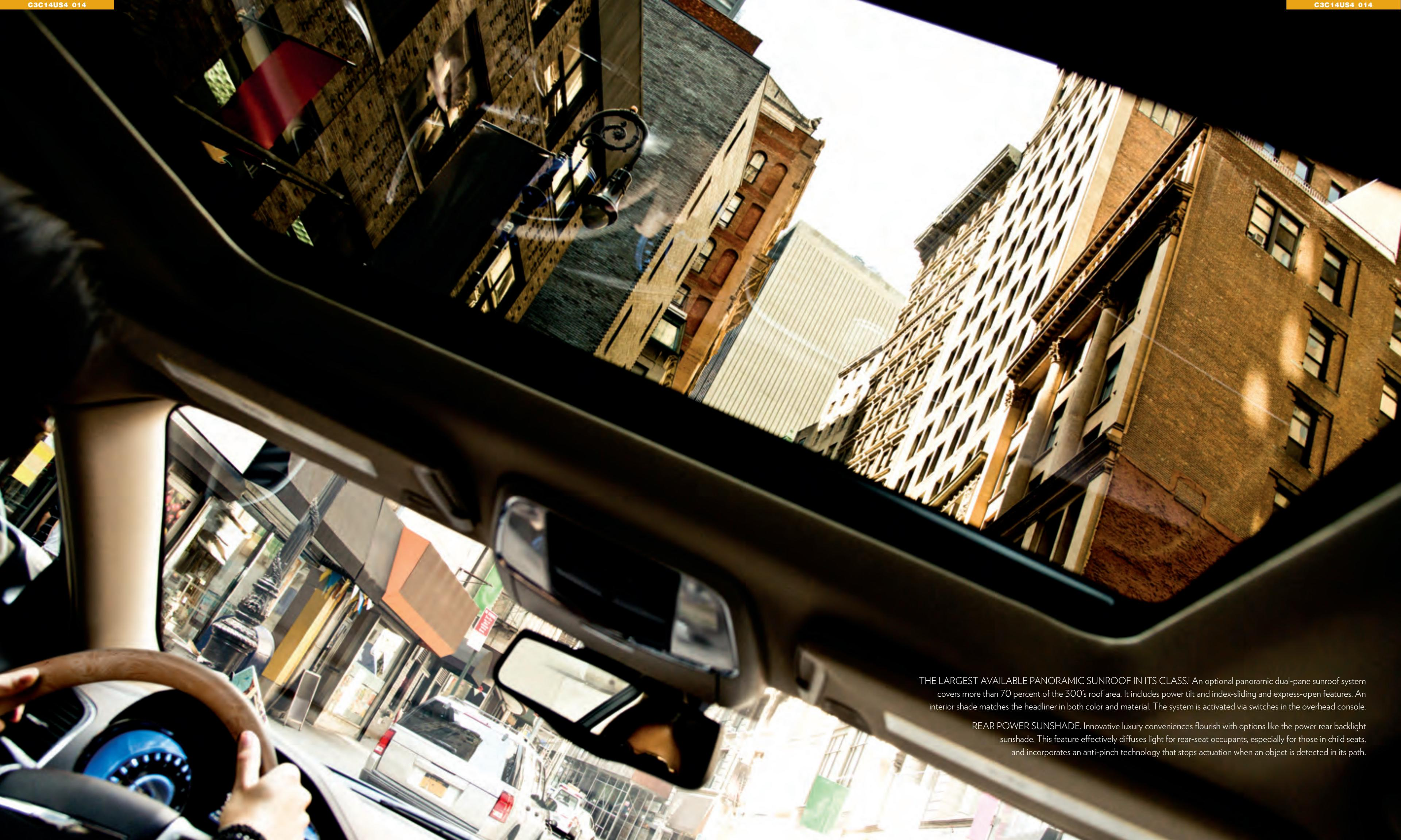
THE LARGEST AVAILABLE PANORAMIC SUNROOF IN ITS CLASS.<sup>1</sup> An optional panoramic dual-pane sunroof system covers more than 70 percent of the 300's roof area. It includes power tilt and index-sliding and express-open features. An interior shade matches the headliner in both color and material. The system is activated via switches in the overhead console.
