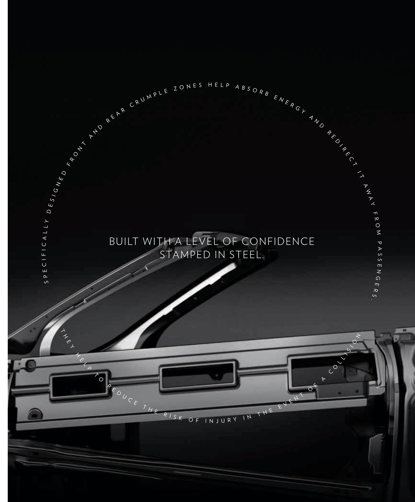
SPECIALLY DESIGNED FRONT AND REAR CRUMPLE ZONES HELP ABSORB ENERGY AND REDIRECT IT AWAY FROM PASSENGERS. THEY HELP TO REDUCE THE RISK OF INJURY IN THE EVENT OF A COLLISION. BUILT WITH A LEVEL OF CONFIDENCE STAMPED IN STEEL.
