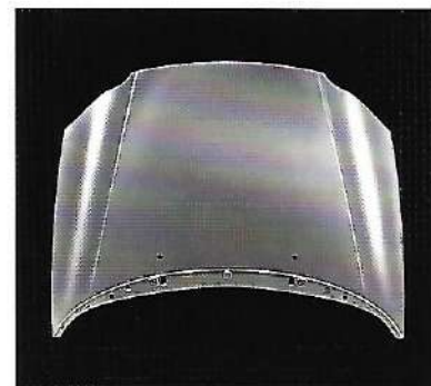
Concorde's hood was Chrysler's first high-volume aluminum exterior body panel.
