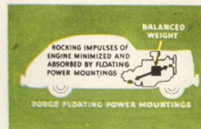
With Patented Floating Power Engine Mountings the engine itself offsets forces which in all motors set up vibration.
