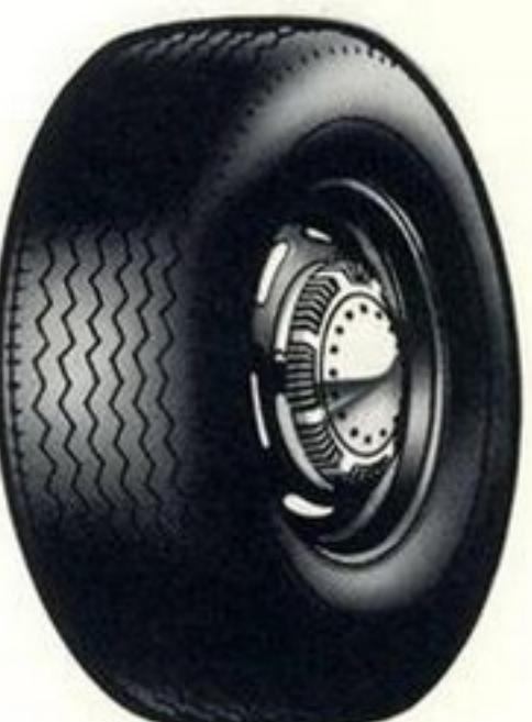
Tires, Aspen Pursuit—FR70 x 14" fabric-belted, radial-ply, high-performance, black sidewall tires, certified for high-speed service are provided with the 318 2-barrel V-8, and 360 2-barrel V-8 engines. These tires are mounted on 14" x 6.0" JJ wheels. GR70 x 15" fabric-belted, radial-ply, high-performance, black sidewall tires mounted on 15" x 7.0" JJ heavy-duty wheels are optional—but are standard with the high-performance 360 4-barrel V-8 engine.
