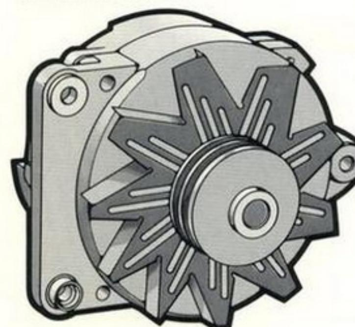
This high-capacity alternator is standard with Monaco Pursuit Packages, optional with Aspen Pursuit Packages. High amperage output was achieved by using more copper in the windings than any previous Dodge alternator. Finned, nickel-plated copper heat sinks keep the diodes operating at proper temperatures even while conducting more current.
