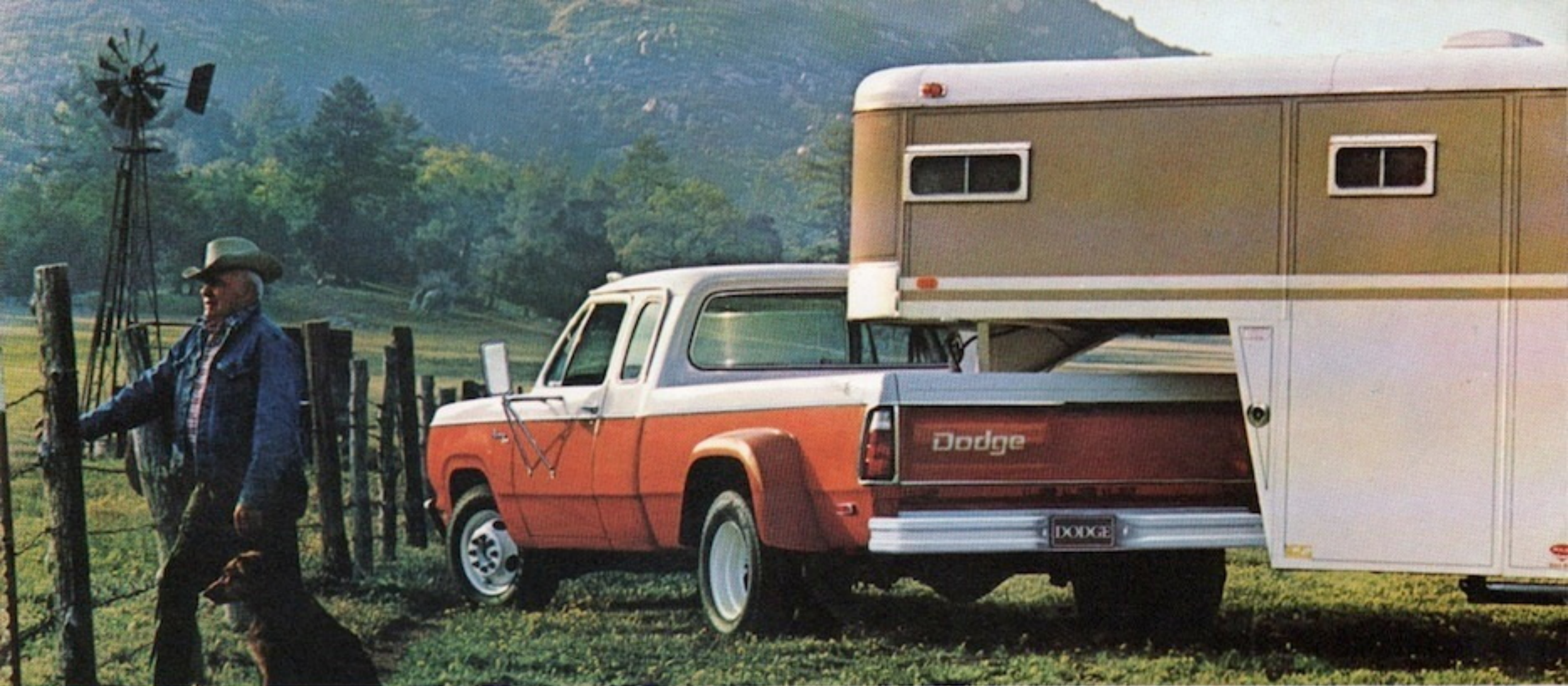
DYNA-TRAC, with dual rear wheels and 10,000-pound GVW. Shown above, D300 Adventurer Sweptline with Dyna-Trac. With optional step-type bumper and rear vision mirrors.
